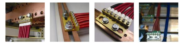
ERICO Connecting, Earthing and Neutral Busbars are used to connect several earthing conductors within a panel and can be used in a variety of different applications including switchgear and control equipment, electrical equipment, for wind and solar power generation and in data centers. This Universal Connecting Bar can be used as a 450A current rating IEC for power distribution.
